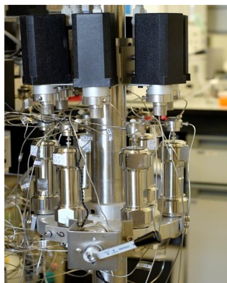
Figure 3.4. A detail of the laboratory scale SMB unit; FlexSMB-LSRE®
