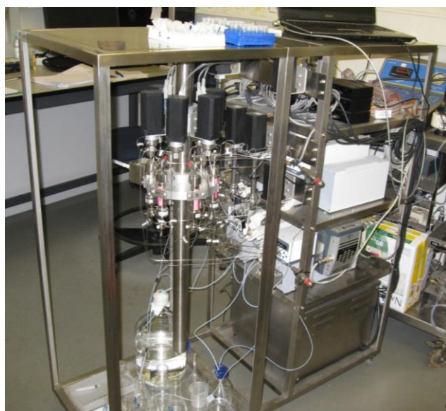
Figure 3.4. A detail of the laboratory scale SMB unit; FlexSMB-LSRE®
