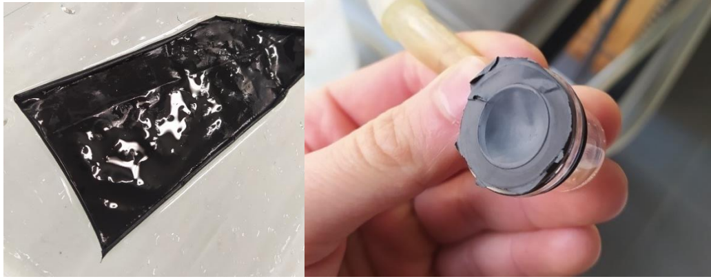
Figure 5. (a) PVP/PVDF@CNTW membrane after molding and coagulation (b) Cut PVP/PVDF@CNTW membrane.
