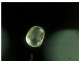
Figure 59. Microscopic images of RAFT imprinted smart hydrogel particles obtained in continuous flow micro-reactor.
