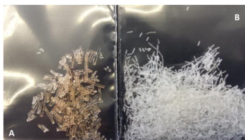
Figure 57. A: RAFT non-linear polymer (CM11). B: FRP non-linear polymer (CM02). (Both synthesis in a MR).
