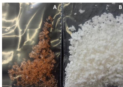
Figure 58. A: Non-linear polymer synthesized on a MR (CM10). B: Non-linear polymer synthesized in a batch reactor (CM05). (Both synthesis using RAFT polymerization).
