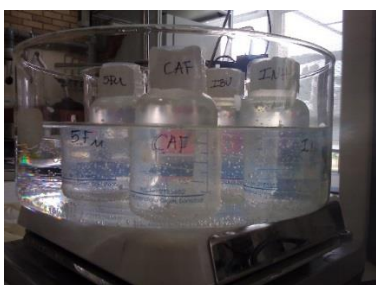
Figure 10. Illustrative image of the controlled drug release tests with PNIPA (thermo-sensitive hydrogel) at 37 °C.
