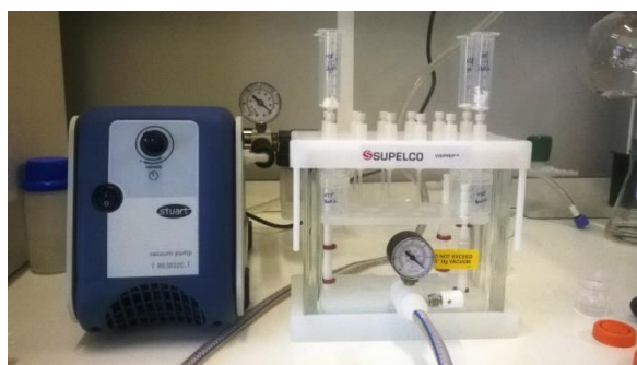
Figure 96. SPE instrument connected to a vacuum pump.
