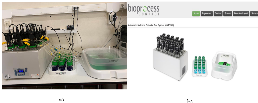
Figure 12: The AMPTS II system by Bioprocess Control. a) a digester unit, a CO 2 absorption bottle, and a volumetric gas measurement unit; b) bioprocess control software.
