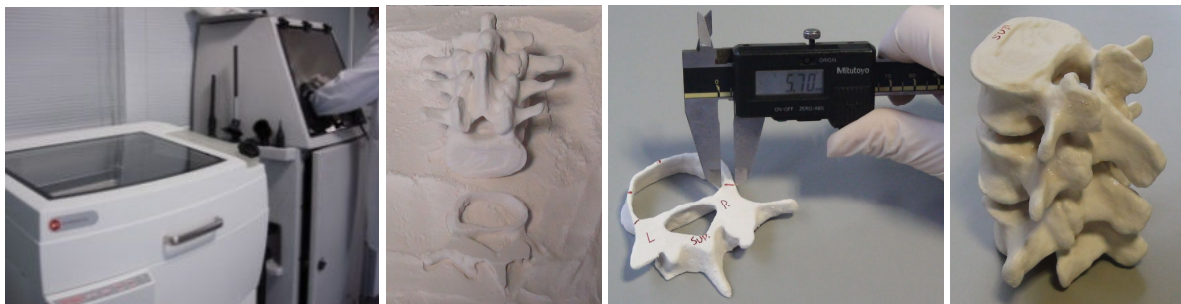
Fig. 2 - ZPrinter and RP experimental methodology used for measure lumbar vertebra segments L4-L2, F52.
