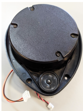
Figure 2.13: The Neato XV-11 laser scanner.
