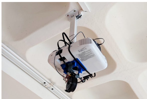
Figure 4.6: Fixing the LiDAR platform to the projector stand.
