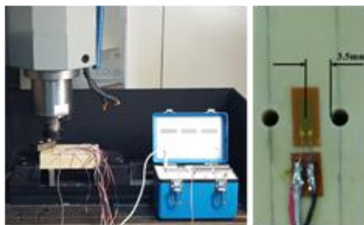
Fig.2 Experimental setup and strain gauges location
