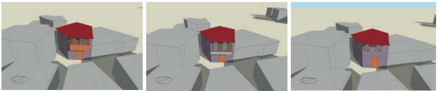
Figure 5. Models of the three scenarios considered in simulations. (left) glazed balcony; (center) balcony; (right) no balcony, small windows.
