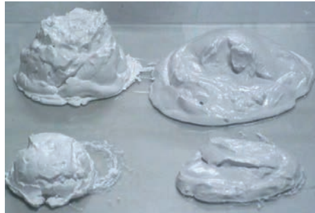
Figure 9. Putty lime with 5 years and 1 month of maturation (Margalha et al. 2011)
