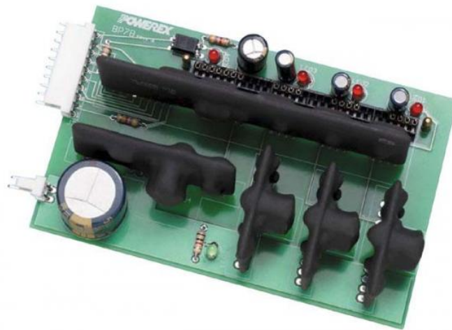
Figure 4.6: BP7B isolation circuit.
