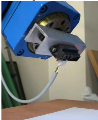
Fig. 13 Sensor positioned in a 45^\circ angle to the obstacle.
