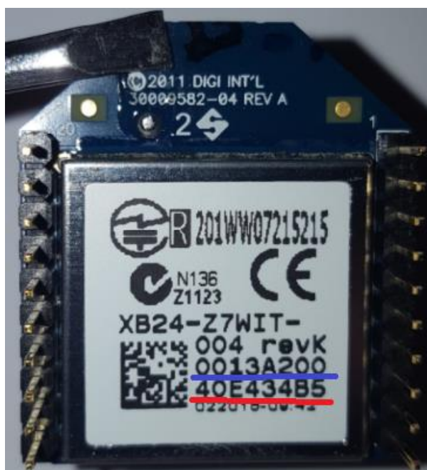
Figura 26 - Endereço DH Destination Address High e DL Destination Address Low.
