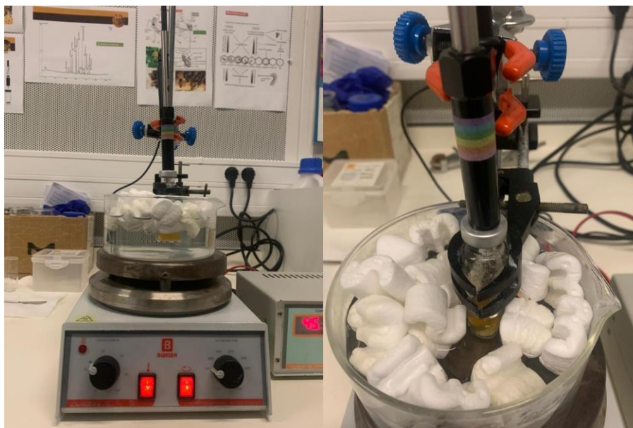
Figure 14. SPME manual system set up for extraction and concentration of volatile compounds from beers.
