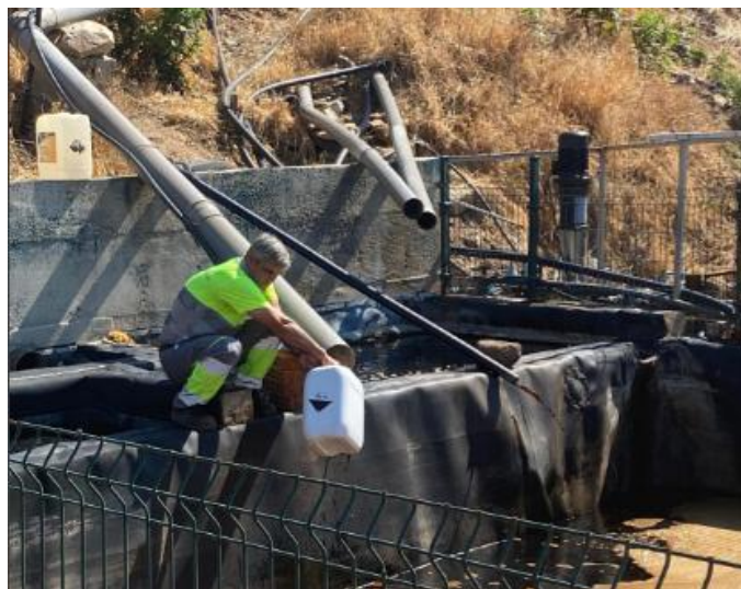
Figure 8. Collection of raw leachate samples for physicochemical analysis.
