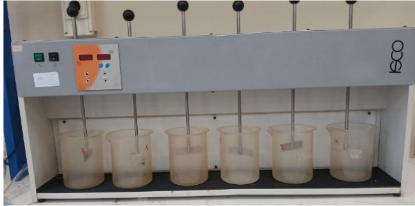
Figure 11. Jar-test apparatus used for assessing coagulant efficiency and floc settling under controlled mixing conditions.
