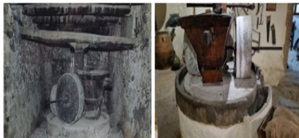
Figure 2.6: The rotary mill animal-powered with larger cylindrical millstones [10].
