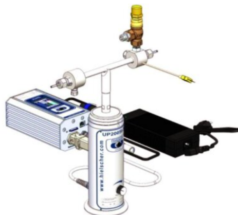
Figure 2.25: real photo of a flow cell ultrasonic reactor[19].
