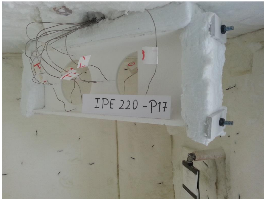
Figure 34: Specimens setup inside the furnace before the test.
