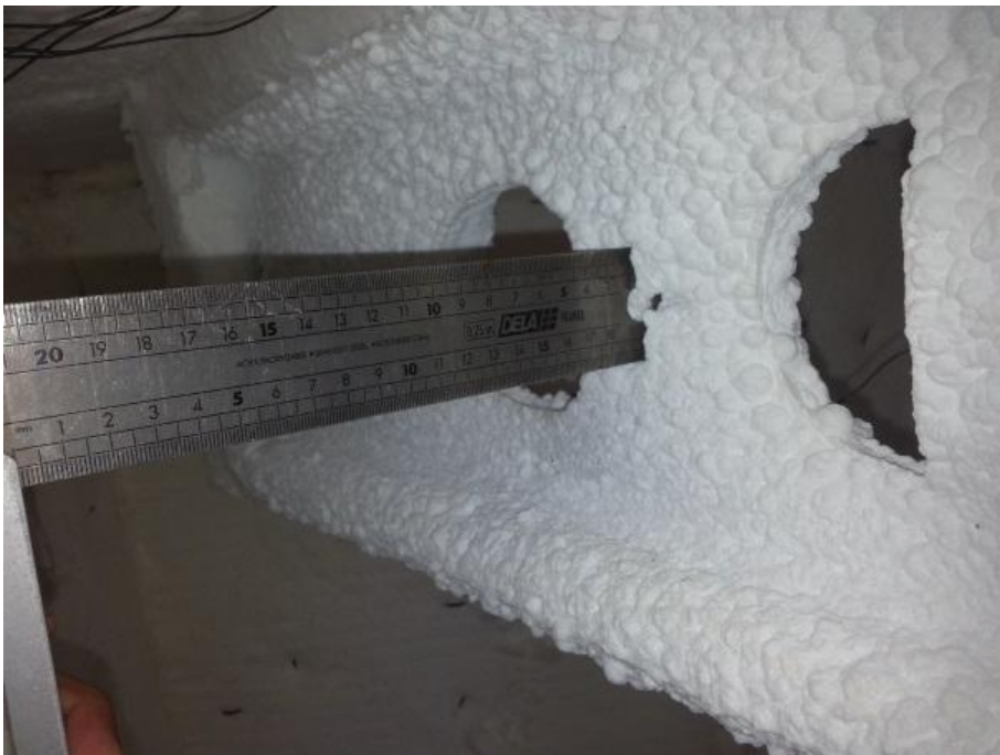
Figure 54: Measured expansion of intumescent char for test P11.
