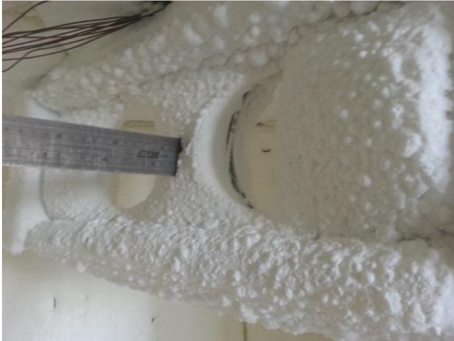
Figure 51: Measured expansion of intumescent char for test P14
