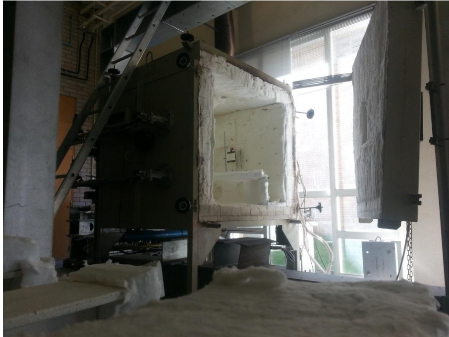
Figure 32: Fire furnace with interior dimensions of 1x1x1 [m 3 ].
