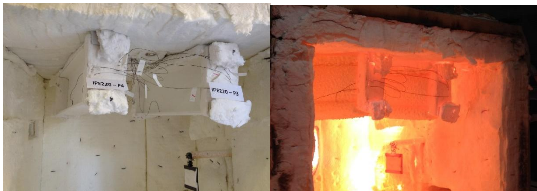
Figure 37 Tests P4 and P3 before and after the test.
