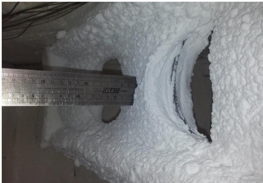
Figure 50: Measured expansion of intumescent char for test P17.
