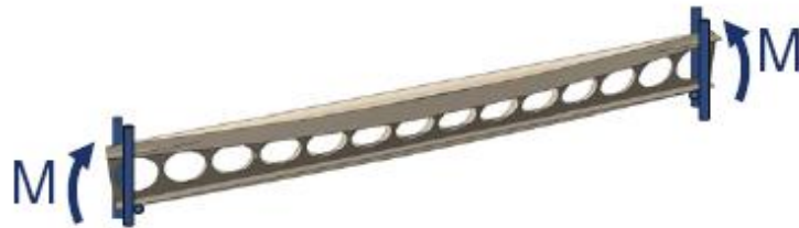
Figure 5: Lateral torsional buckling failure of a cellular member loaded by a bending, [9].
