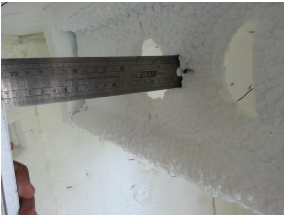
Figure 51: Measured expansion of intumescent char for test P14
