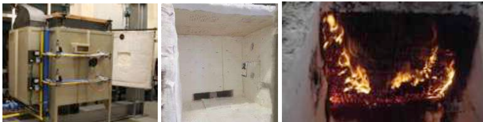
Figure 3 – Fire resistance furnace in laboratory, before and after the test
