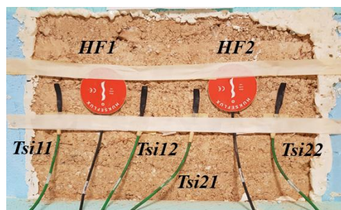
Figure 4: Placement of the sensors in the case of Soil S2 : heat flux sensors HF1 and HF2 and inner surface temperature thermocouples Tsi11 , Tsi12 , Tsi21 and Tsi22 .
