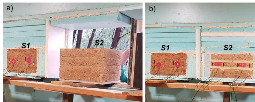
Figure 3: Experimental procedure for the 2 nd measurement period: a) placement of sample S2 ; b) instrumentation of S1 and S2 .
