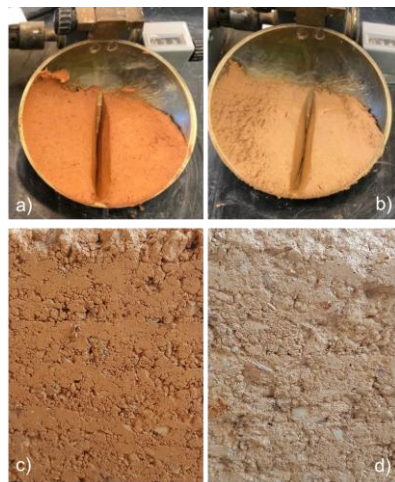
Figure 2: Liquid limit (LL) test: a) Soil S1 and b) Soil S2 ; Manufacturing process: c) Soil S1 and d) Soil S2 .
