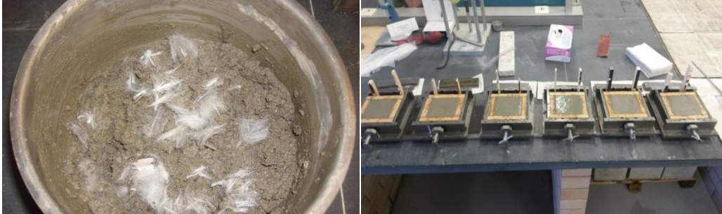
Figure 1: Preparation of concrete samples with PP fibres.
