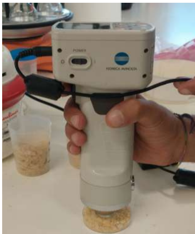
Figure 11. Use of a Konica Minolta Colorimeter for Color Measurement of Sample Material
