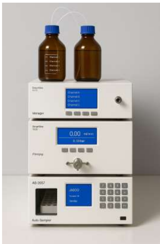
Figure 16. Configuration of the HPLC System Comprising a Knauer Smartline 1000 Pump, Smartline Manager 5000 Degasser, and Jasco AS-2057 Auto-Sampler
