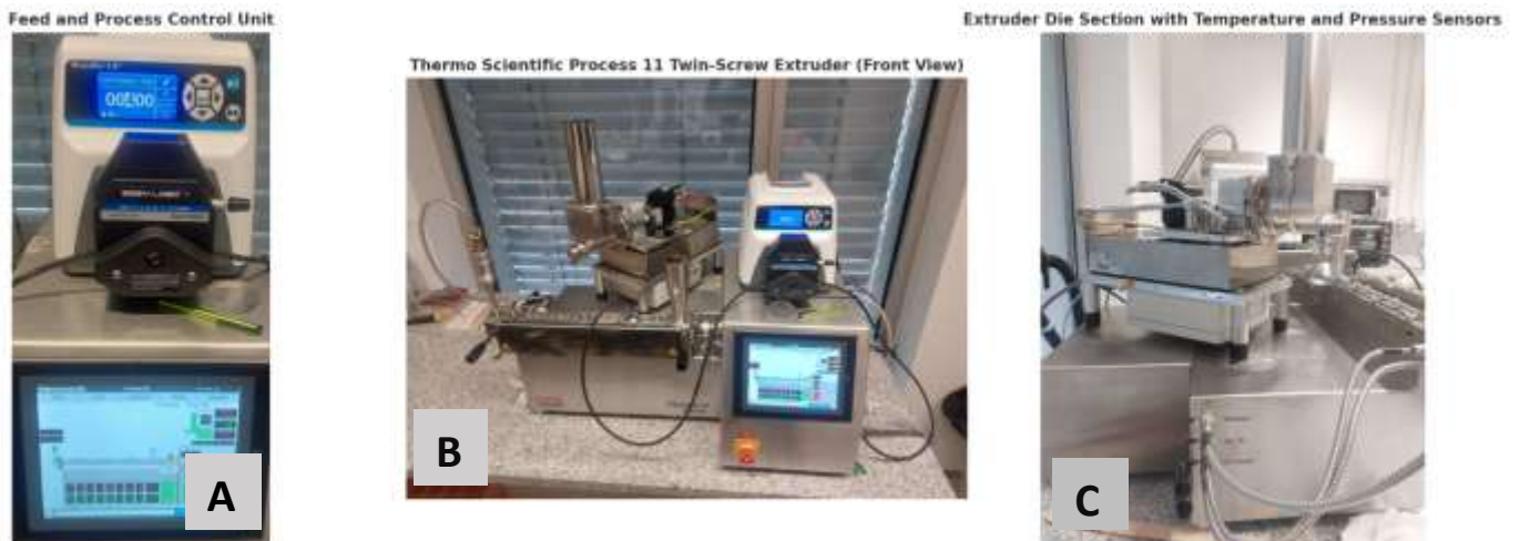
Figure 9. A: Control unit. B: Front view of twin-screw extruder. C: Die section with temperature and pressure sensors.
