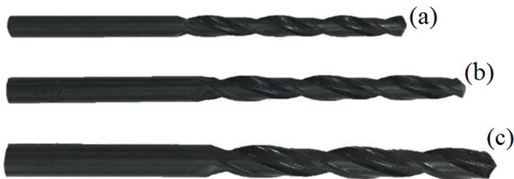
Fig. 2 - Drill bit diameters used in this study: (a) 4 mm, (b) 5 mm and (c) 6 mm.
