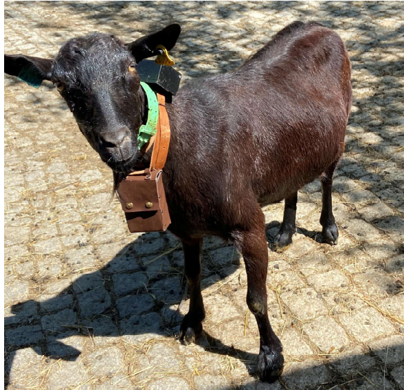
Fig. 2: Device fitted to the animal. In the image you can see the arrangement of the device on the animal, where the top supports all the modules and sensors and the bottom the feeding system. This distribution ensures that the bottom part counterbalances the device so that the top part is always on top of the animal.
