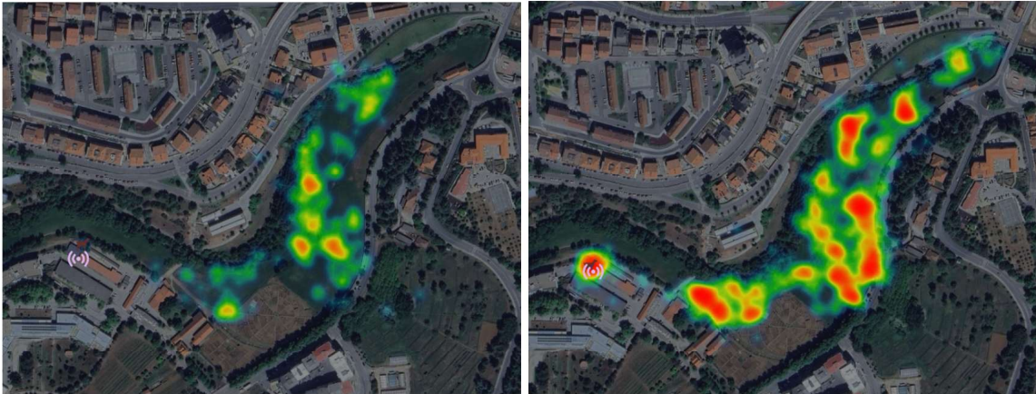
Fig. 3: Heat maps generated by Grafana. These heat maps were generated based on two days of grazing recorded by the system. In both cases, there is a distribution of green and red spots which indicate the areas preferred by the animals (the red ones indicate longer stays by the animals).
