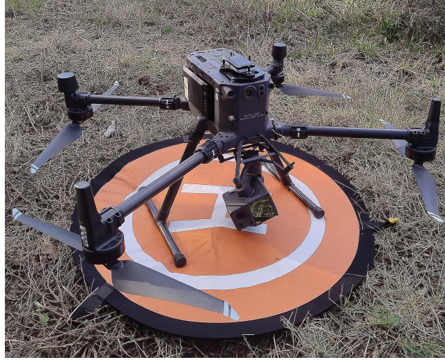
Figure 3.2: UAV-based LiDAR set employed in this study (M300 RTK + L1 Zenmuse).
