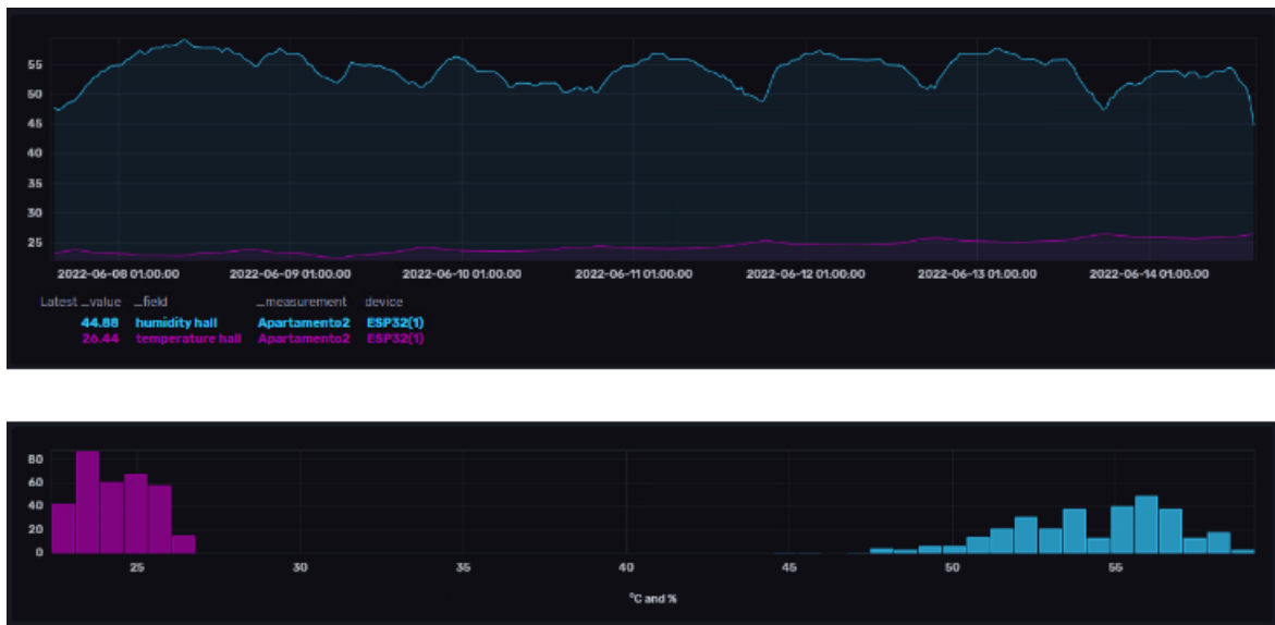
Figure 5.6: Humidity and temperature of the DHT11 sensor for one week.
