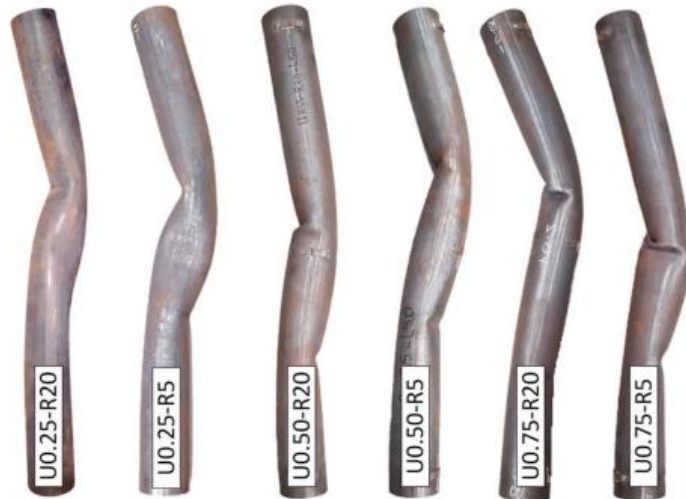
Figure 8 – Failure mode of the UHSS tubes in the fire tests. [3]
