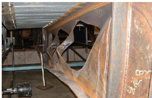
Figure 4: Web-post lateral-torsional buckling, [2].
