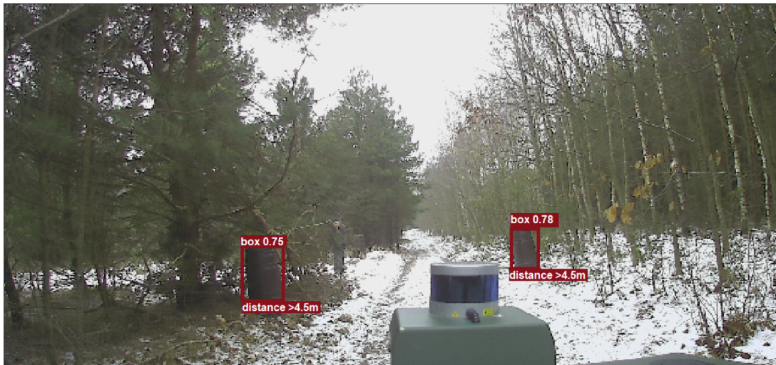
Fig. 9. Examples of detected objects using fused model in operational environment with assigned estimated distance.
