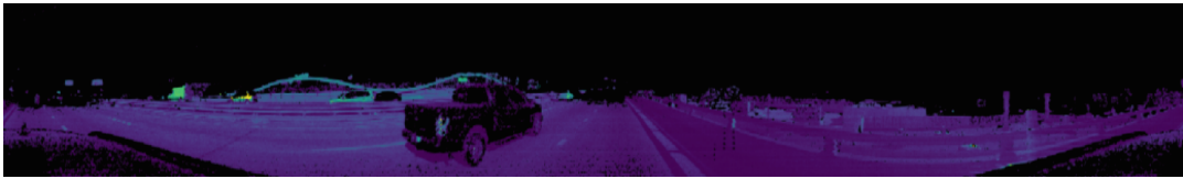
Fig. 10. Example of flat view from Ouster OS1-128 LiDAR point cloud surfaces.
