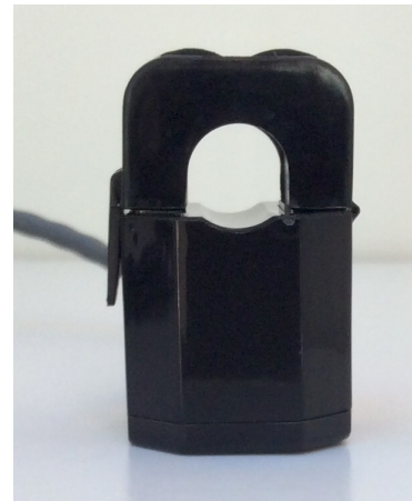
Figure 4.3: IoTaWatt's current transformer. [63]
