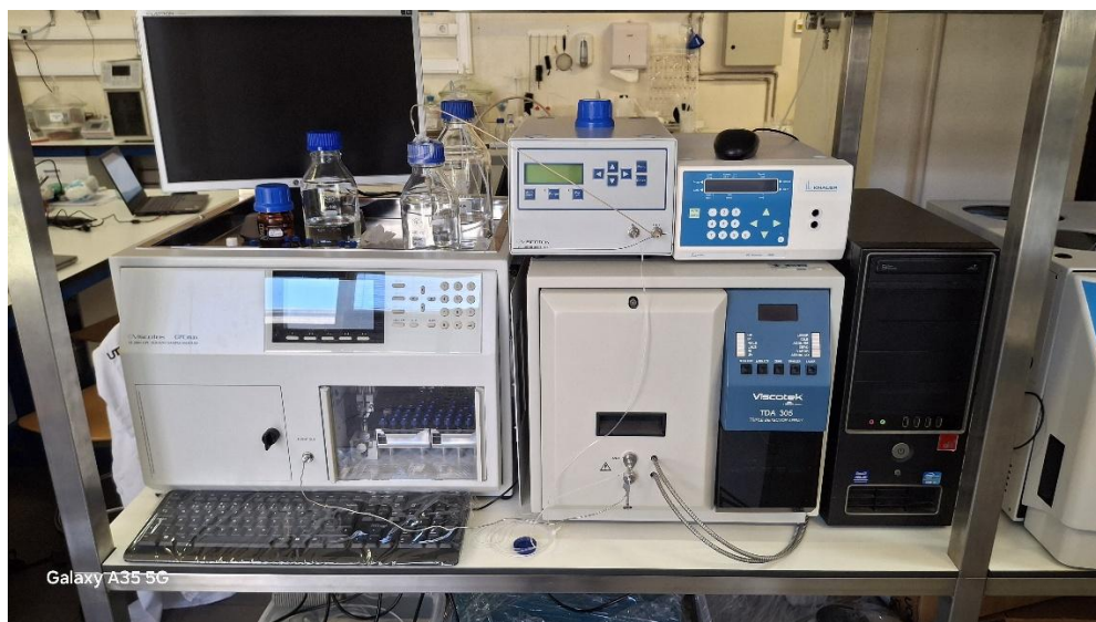
Figure 6: GPC system with RI/LALS/RALS detection (DMF-based) used for oligomer analysis
