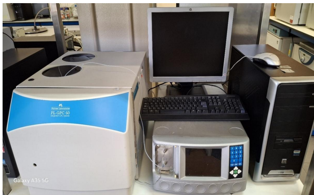
Figure 7 : GPC system with RI/LALS/RALS detection chloroform-based) used for PHB oligomers and polyurethane analysis
