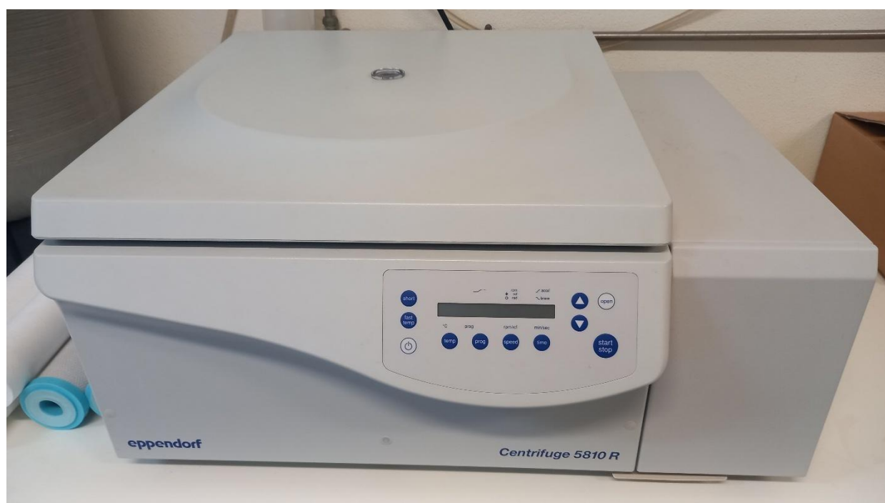
Figure 8: Large-capacity digital centrifuge (Eppendorf 5810 R) used for phase separation and purification of PHB oligomers and polyurethane precipitates during sample processing.
