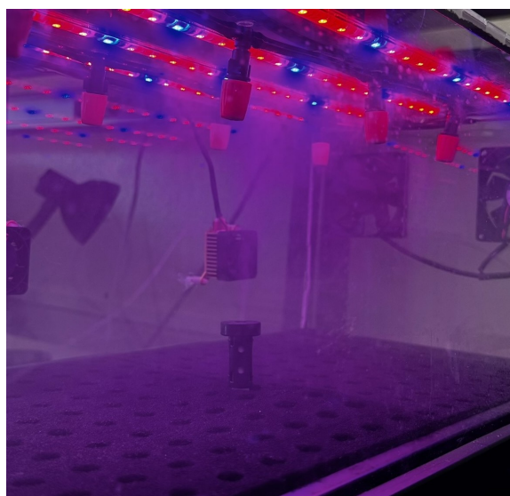
Figure 5.6: Air humidity tests using atomizers.
