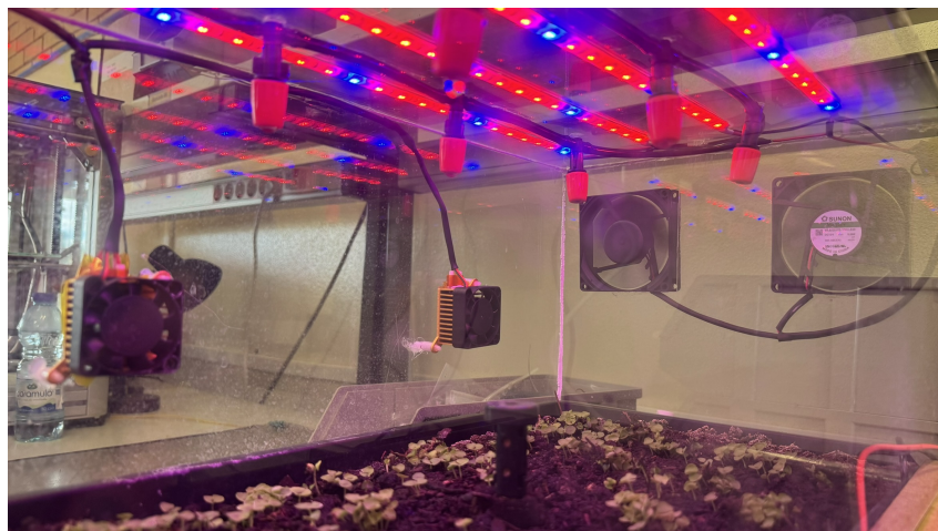
Figure 5.5: Heating tests with thermal pads attached to heat sinks.
