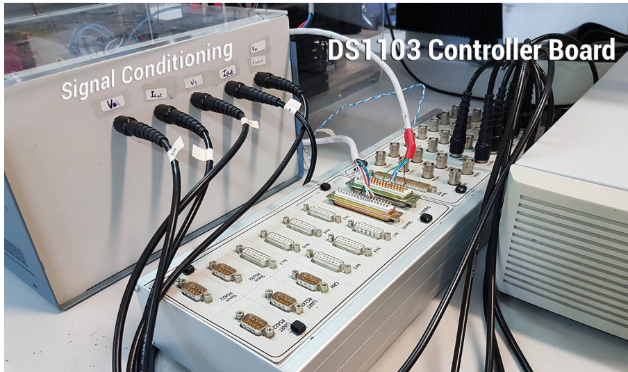
Figure 4.11: DS1103 Controller Board and outputs from signal conditioning module.
