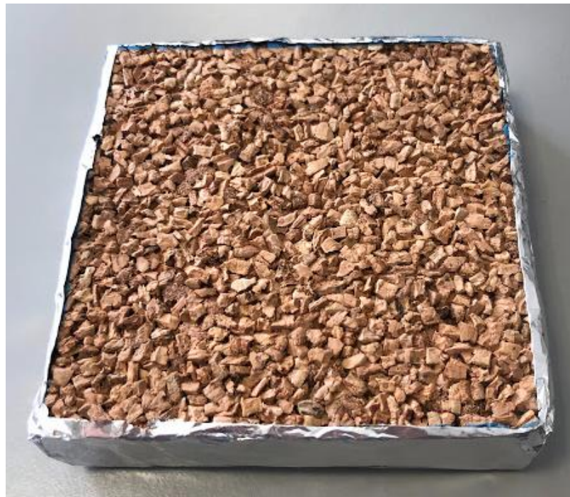
Figure 15: Sample wrapped in aluminium foil before testing.
