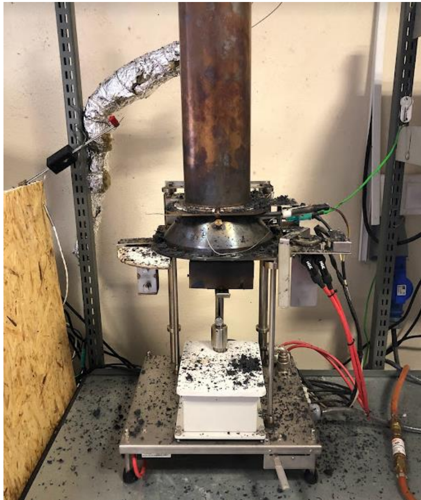
Figure 31: Working environment after testing a TDI sample with 20% expandable graphite.
