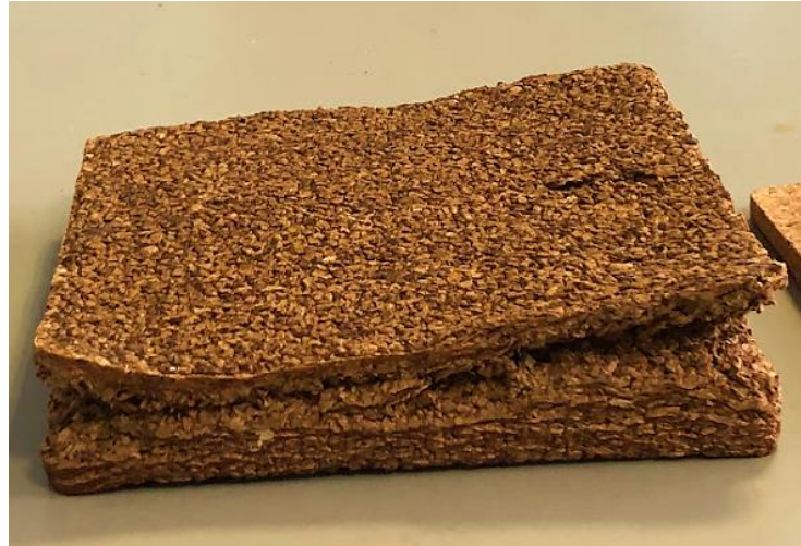
Figure 20: Panel faulty due to excessive pressure applied
