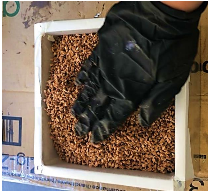
Figure 8: Manual levelling the compound.
