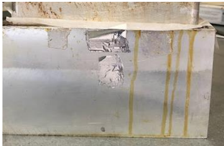
Figure 21: Mould with traces of run-off resin.
