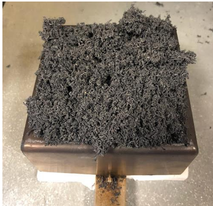
Figure 40: MDI specimen with 10% of EG after a test carried out at 50kW/m 2 .
