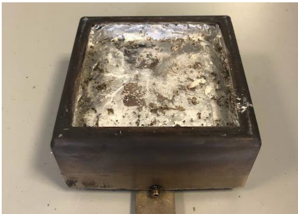
Figure 30: A specimen without flame retardant after the end of the test.
