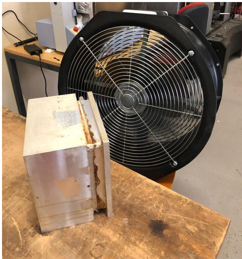
Figure 12: Cooling the mould.
