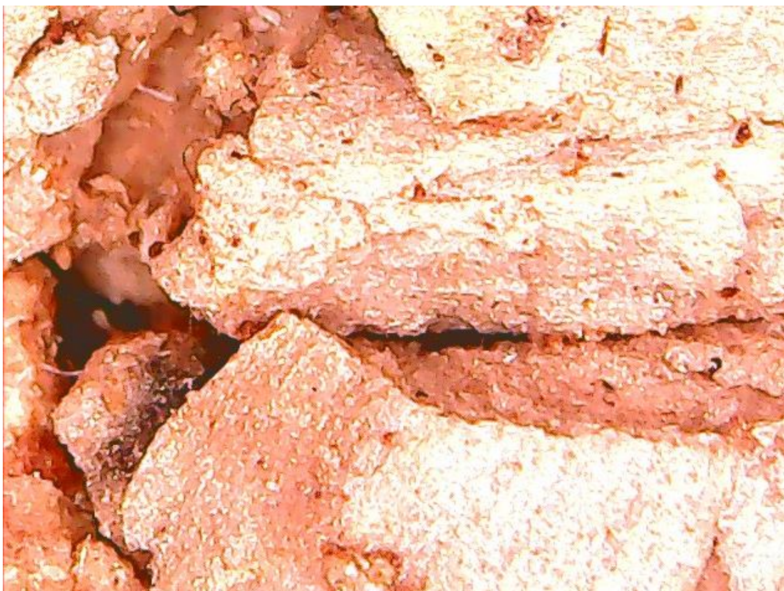
Figure 25: Agglomerated cork with 0% EG magnified at 200x.
