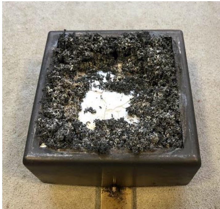
Figure 39: MDI specimen with 5% of EG after a test carried out at 50kW/m 2 .
