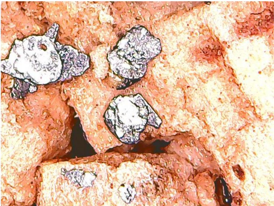
Figure 27: Agglomerated cork with 10% EG magnified at 200x.
