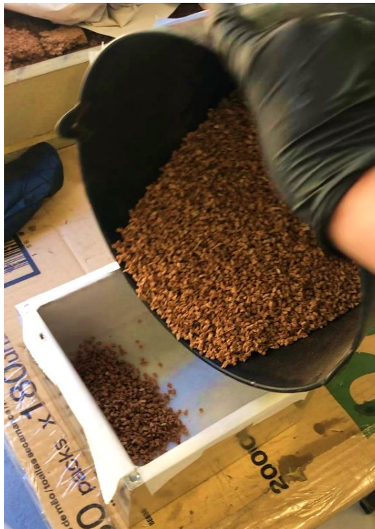
Figure 7: Mould filling for making an agglomerated cork.
