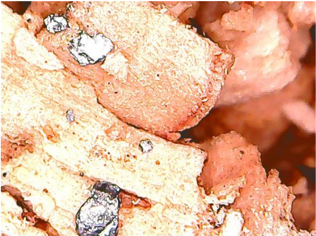
Figure 26: Agglomerated cork with 5% EG magnified at 200x.
