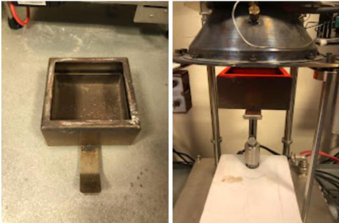
Figure 17 (a and b): sample holder empty and positioned for the baseline collection, respectively.
