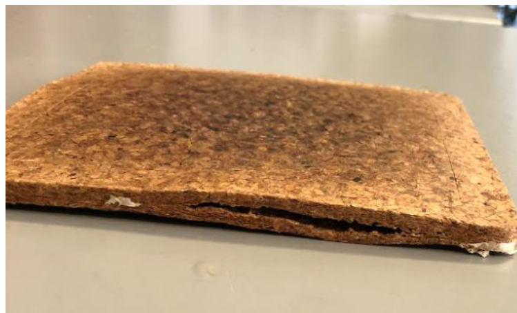
Figure 22: Extremely compacted agglomerate with a rupture inside.
