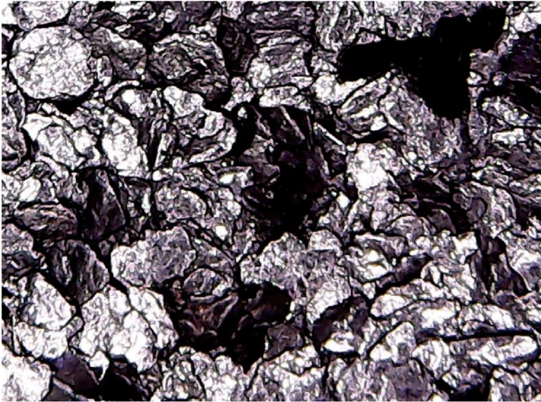
Figure 33: EG before being exposed to heat (200x zoom).
