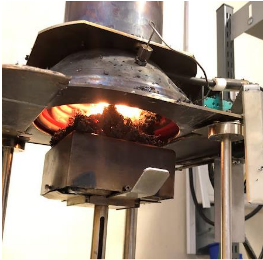
Figure 32: TDI sample with 20% expandable graphite touching the cone during a test.
