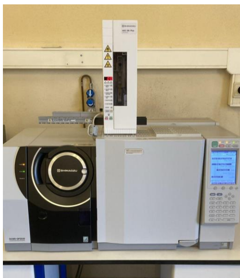
Figure 9 - Gas chromatography - mass spectrometry equipment utilized. Source: Author, 2023.
