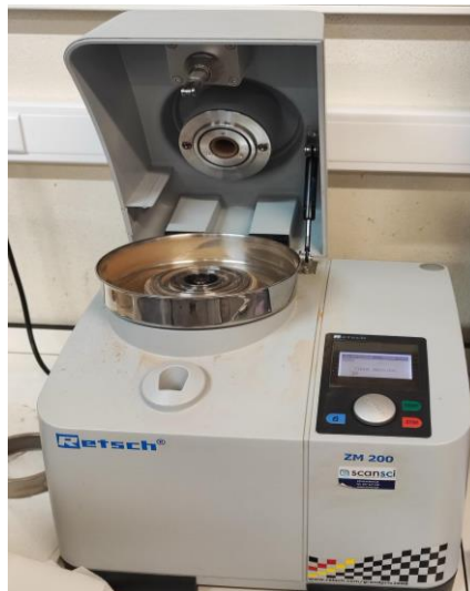
Figure 7 - Grinding Equipment Source: Author, 2023.
