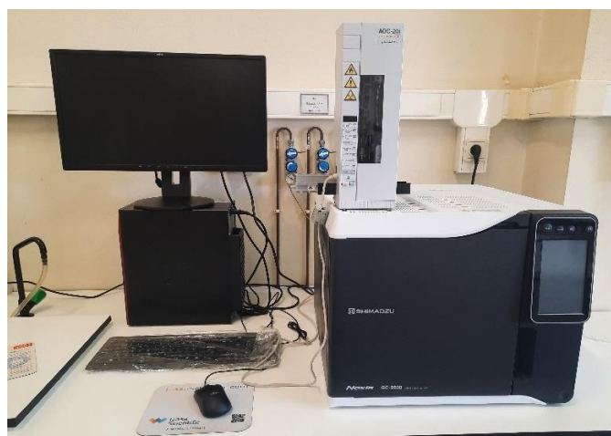
Figure 10. GC-FID equipment used for FAME content analysis in biodiesel sample.
