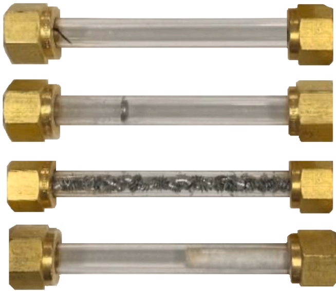
Fig. 12. Test samples for tube insertion. Sequentially arranged as: Absence of insertion, stainless steel disc, compressed shavings, and felt, adapted from [71].
