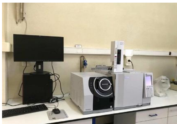
Figure 12. GC-MS equipment used for the analysis of volatile molecules
