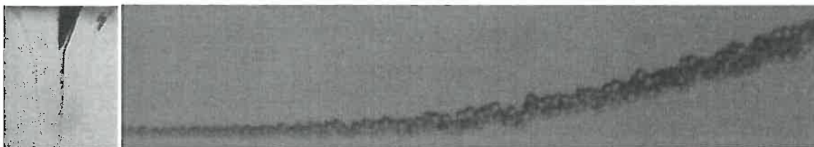
Fig. 1. (Left) Precursor jet of PDMS particles. (Right) Stream of droplets, about 5 microns in diameter, behind the nozzle.
