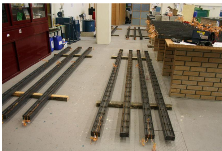
Fig.4 Specimens prepared for casting phase.
