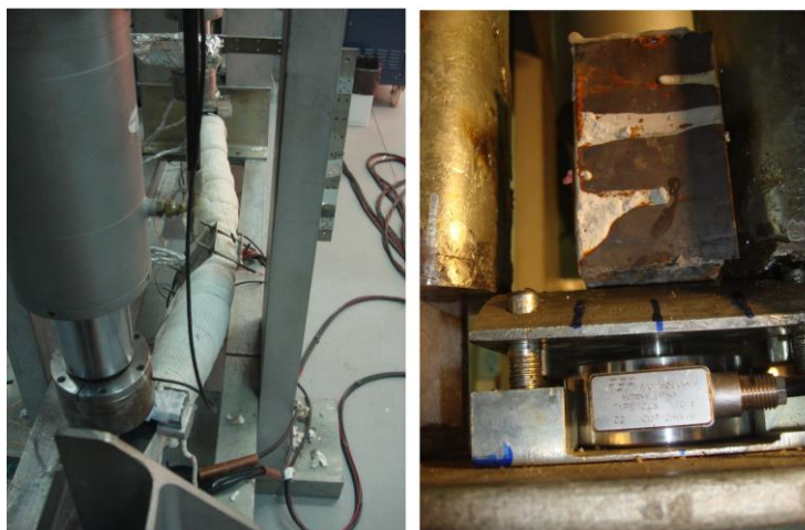
Fig.3 Load applied by the hydraulic jacks (left) and testing supports with load cell (right).
