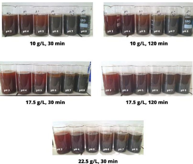
Fig 8: Visual aspect of samples for pH variation in 10, 17.5 and 22.5 g/L coagulant and settling time of 30 and 120 minutes
