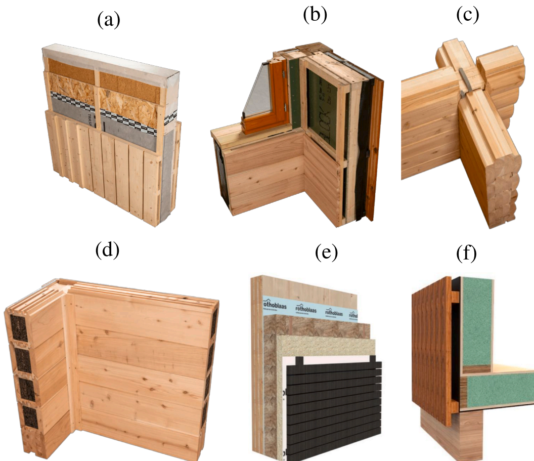
Fig. 2. Methods to assemble building elements in timber construction: (a) LTF wall with wood fibre cavity insulation; (b) Post-and-beam structure with a timber frame infill wall; (c) Wall junction with laminated logs; (d) Prefabricated timber system with cork core insulation; (e) CLT wall with double insulation; (f) Prefabricated structural insulated panels with foam insulation sandwiched between wood-based boards; Photos (a), (b), (c), (d) by Rusticasa [27]; Photos (e), (f) by New Edge [28].
