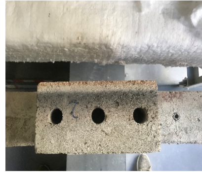
Figure 8: CEBs after expose to the fire.
