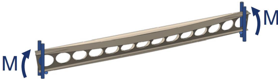
Figure 6. Lateral–torsional buckling failure of a cellular beam loaded by a bending moment, [9].
