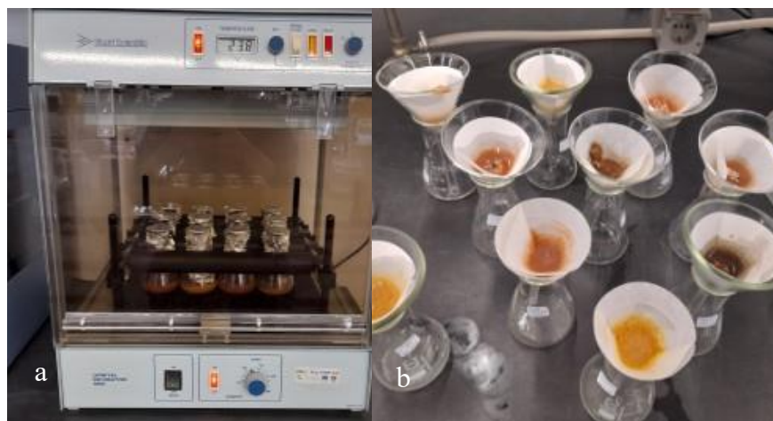
Figure 8. Orbital shaker set for 120 rpm (a), sample filtration with Whatman #3 paper in glass wholes to retrieve the filtrate (b).
