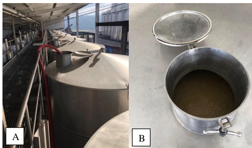
Figure 16: A - Stainless steel tanks in the fermentation process. B - White must fermenting.
