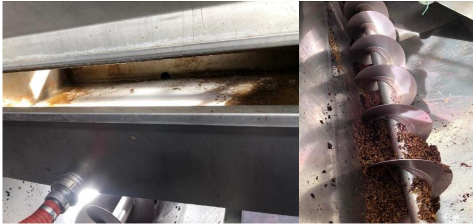
Figure 15: Separation of the liquid part (must) from the solid part (pomace) after pressing.
