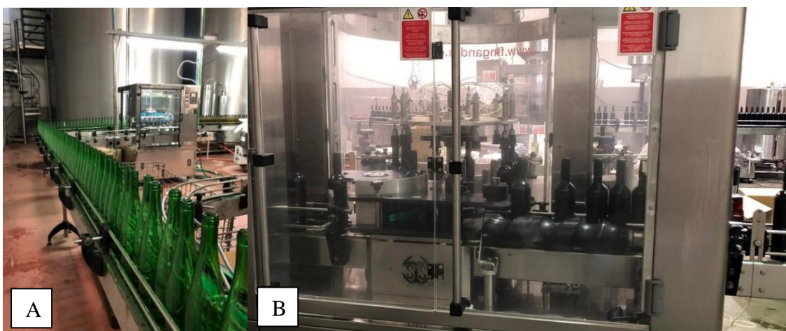
Figure 17: A - Glass bottles in alignment process for rinsing. B - Glass bottles with corks in the encapsulation process.
