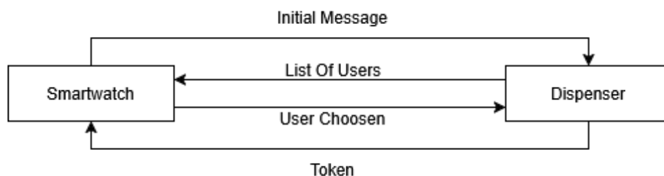
Figure 4.4: Messages exchanged between the smartwatch and the dispenser
