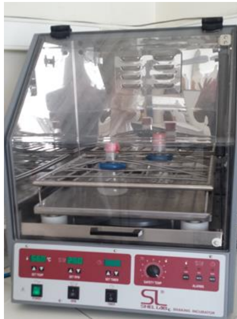
Figura 2.1: Incubadora com agitação (modelo ShellLAB, Shaking Incubator, marca Sheldon Manufacturing, INC).
