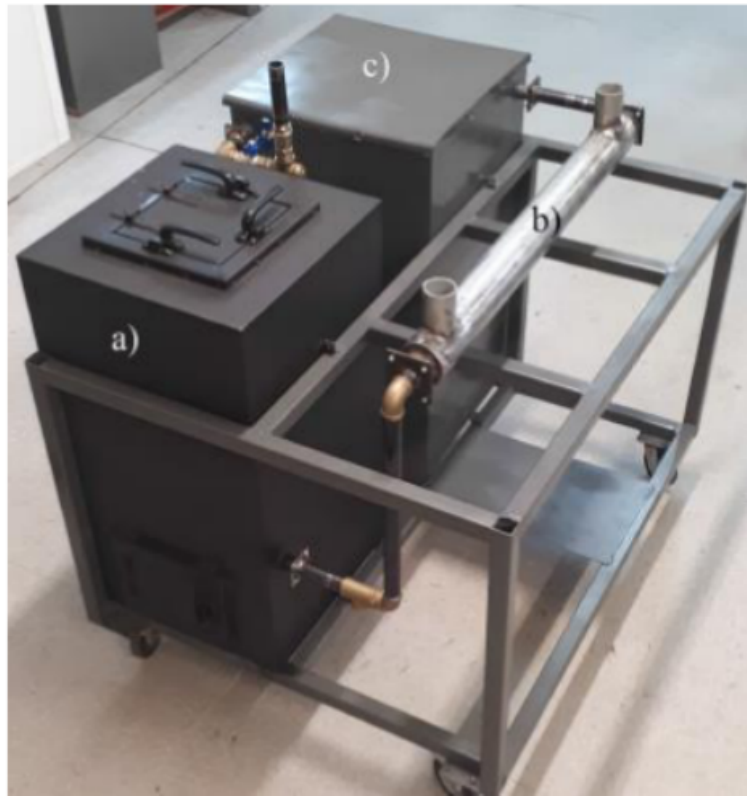
Figure 3.3: Prototype of the gasification system to supply the Campeon motor pump with syngas
