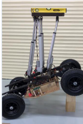
Figure 2.10: Stewart Platform on mobile robot for self stabilization [34]
