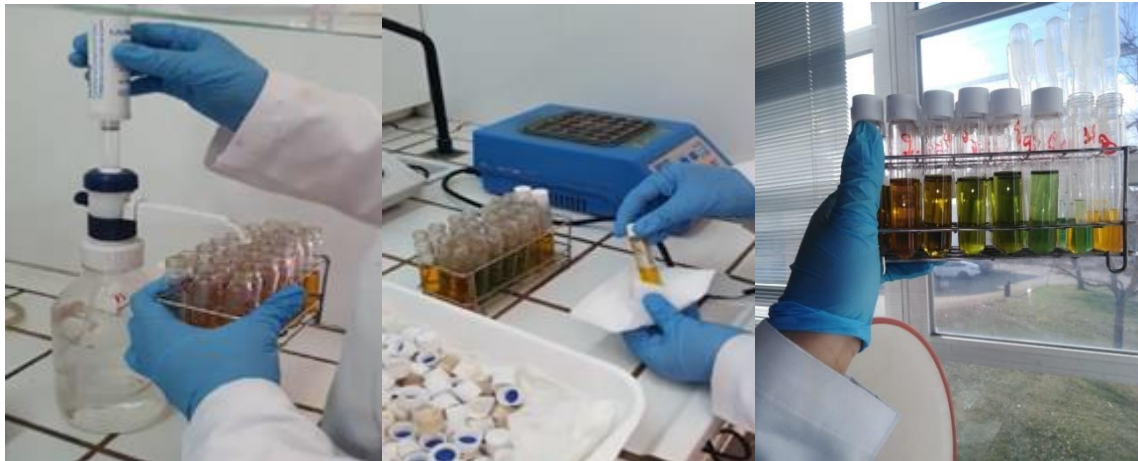
Figure 12: The experimental steps of the COD Removal test
