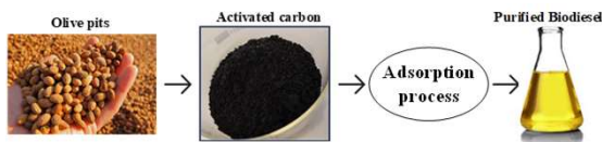
Fig. 2. Activated carbon production and adsorption.
