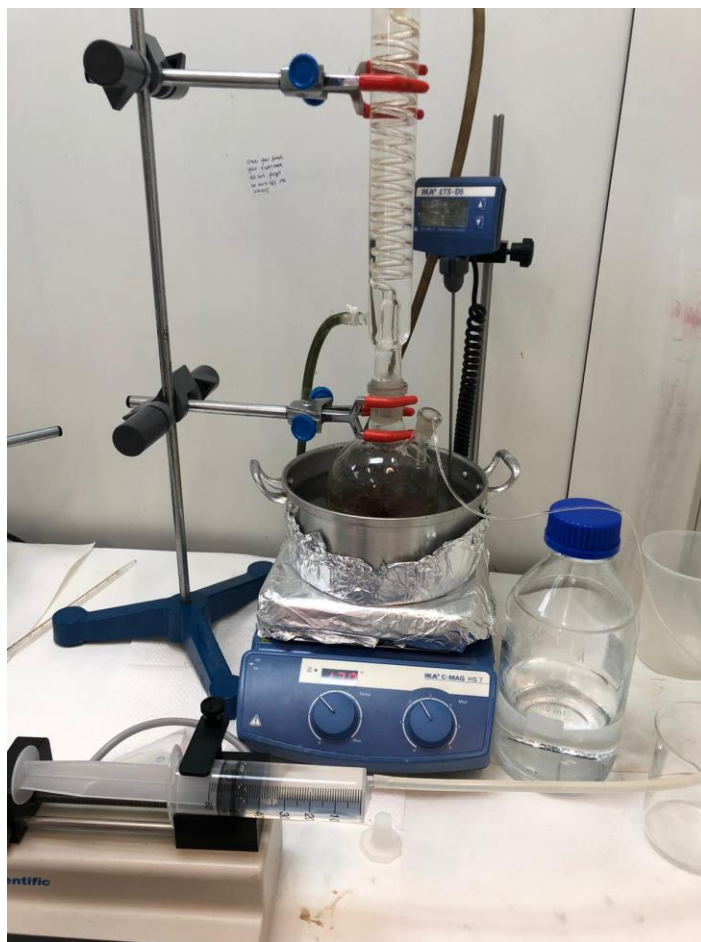
Figure 5: System used to drop the NaOH solution into the MNPs suspension
